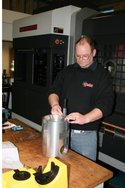
A Norbar Torque CNC Setter inspects a component machined on one of the company's two new Mori Seiki NTX mill-turn machines
